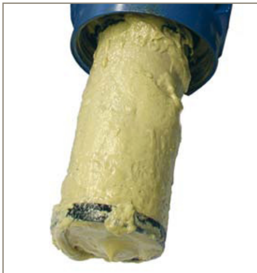
Typical contamination removed by a railway industry type TFGE / TFHE compressed air filter
